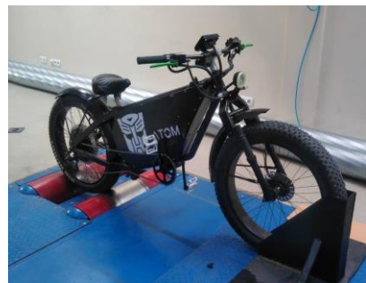
Fig. 1. Light two-wheeled electric vehicle powered by 3 kW BLDC motor and classical bicycle pedals
