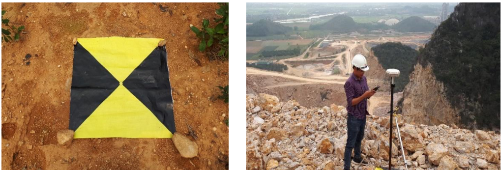
Fig. 2. GCP marks and their coordinates measured by GNSS/RTK
