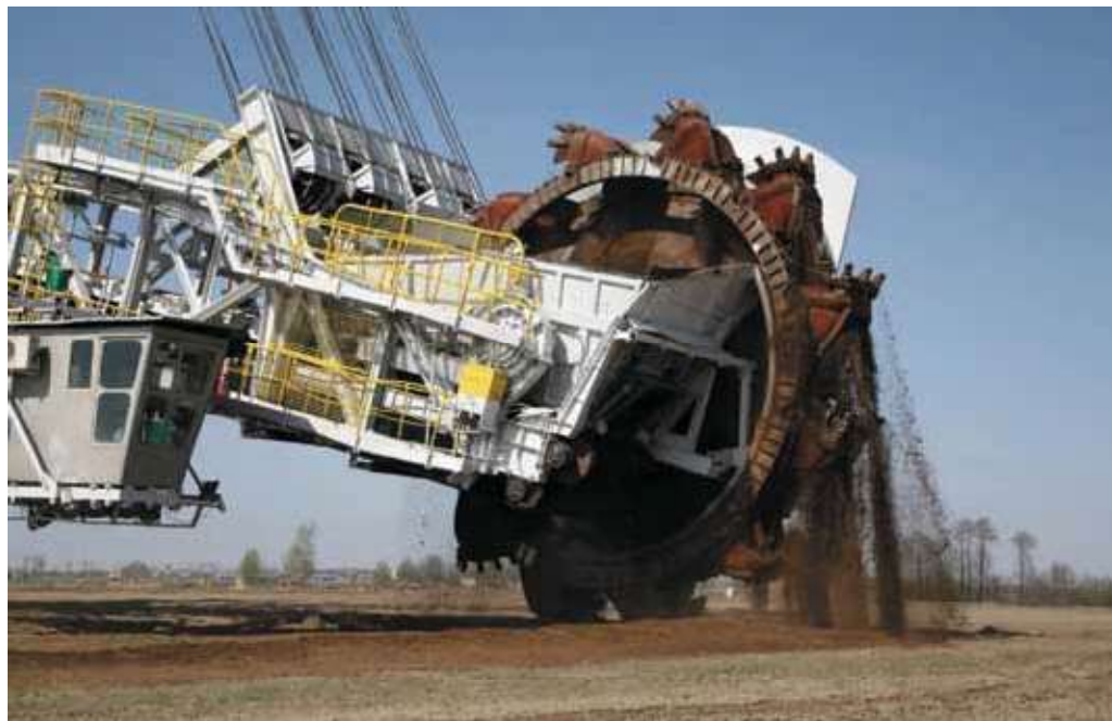
Fig. 4. Bucket wheel of the KWK 1500s BWE in Tomislawice open pit mining plant in PAK KWB Konin S.A. [Photo. P. Ordan]
