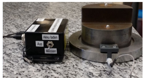
Fig. 3. Flowability sensor and the wireless system
