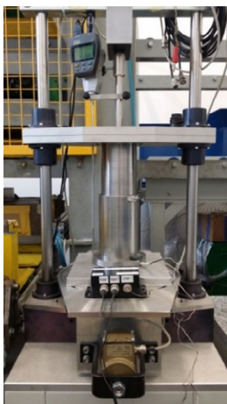
Fig. 5. Pressing machine, sensor and wireless system
