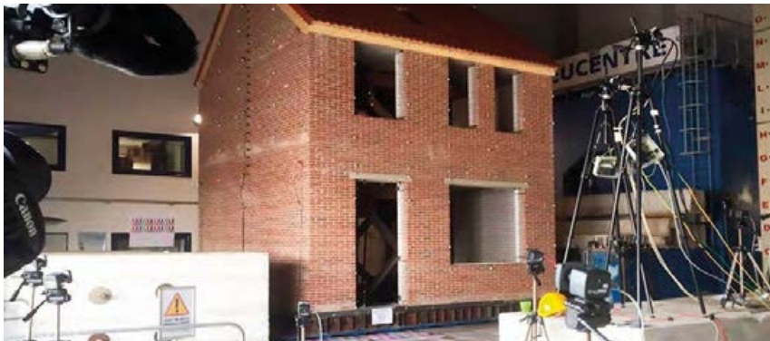
Fig. 14. Shaking table test on a typical Dutch house in Pavia, Italy, 2015
