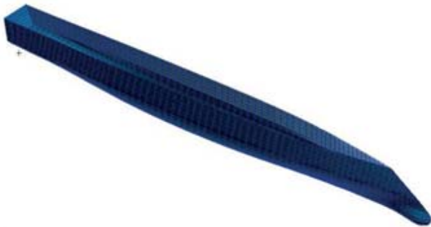
Fig. 4. Sketch of panel model and the hydrodynamic grid ( \alpha=60^\circ , \beta=10^\circ )
