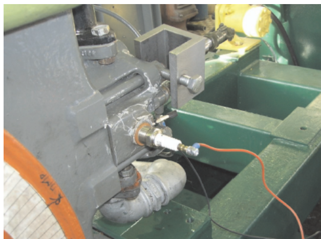
Fig. 4. Langmuir probe mounted in the cylinder of a Farryman Diesel D10 engine Rys. 4. Sonda Langmuira umieszczona w cylindrze silnika Farryman Diesel D10
