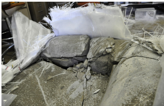
Fig. 10. Grout bag cut open to show failure surfaces
