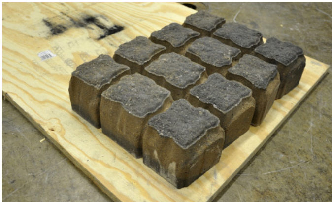
Fig. 11. Photograph of four sets of concrete pavers used to simulate a mine roof
