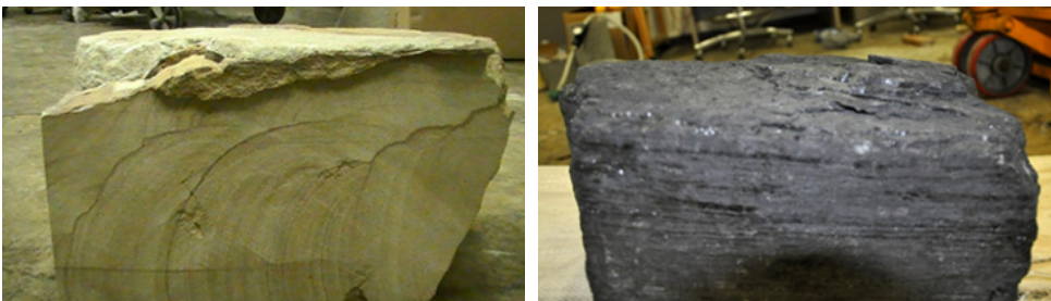
Fig. 6. "Rough" surface of sandstone and coal blocks
