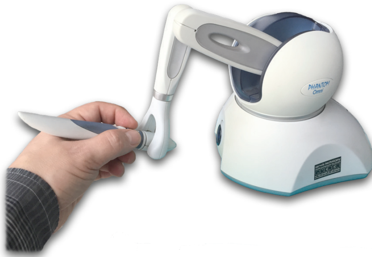
Fig. 5. The PHANTOM Omni haptic device
