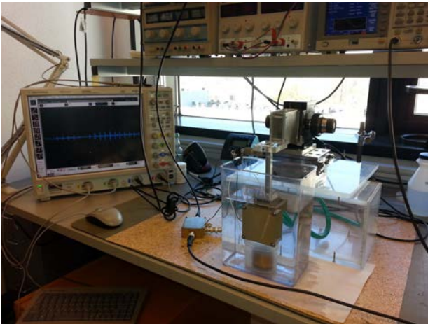
Fig. 5. Experimental setup (real view) for measuring the transmitted and back-scattered field acoustic field.
