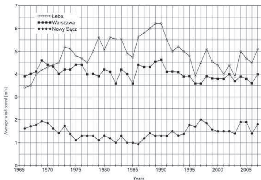
Figure 1. The many years variability of annual average wind speed for Łeba, Warsaw, Nowy Sącz from 1966 to 2007 (according to the data of IMGW Warsaw).
