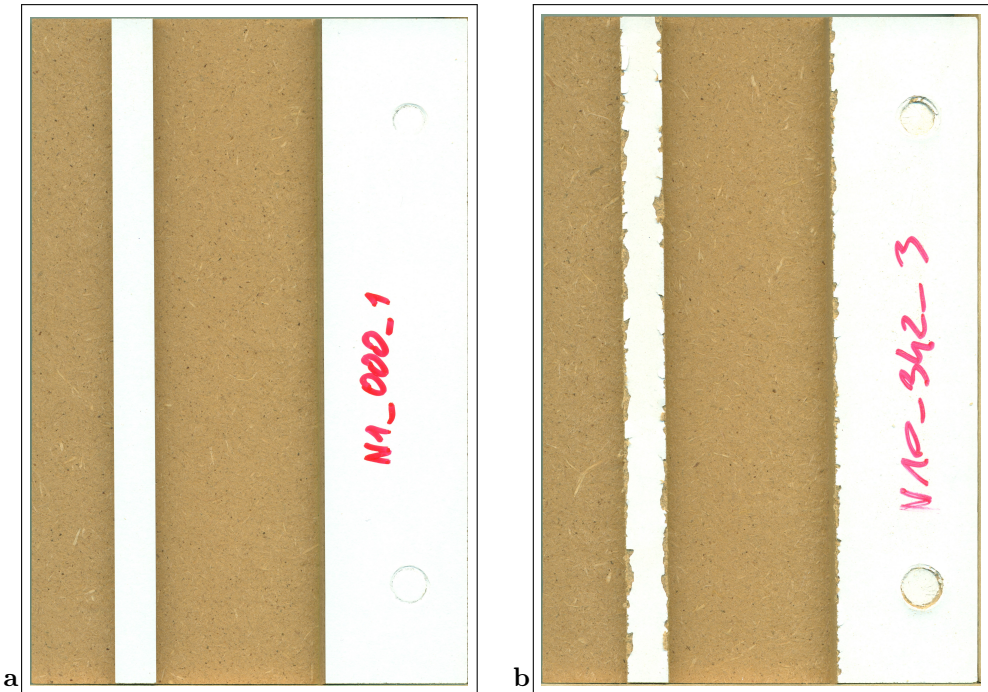
Fig. 1. Examples of scanned samples: (a) milled with a new tool; (b) milled with a very used-up tool.
