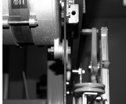
Fig. 5. Motor attached with insulating pads made of 2 mm thick polyurethane
