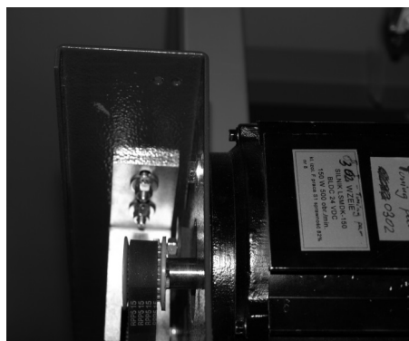
Fig. 4. Way of mounting the motor to the main carrier without insulating pads
