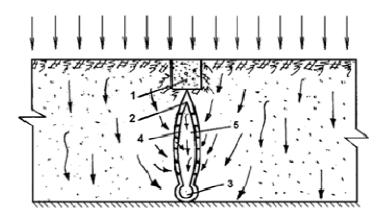
Fig. 4. Cross section of the combine three-tier drainage
