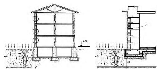
Fig. 5. Plan of the combined three-tier drainage in the building foundation
