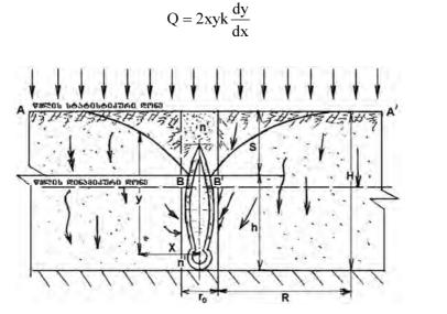
Fig. 6. Calculation plan of the combined three-tier drainage
