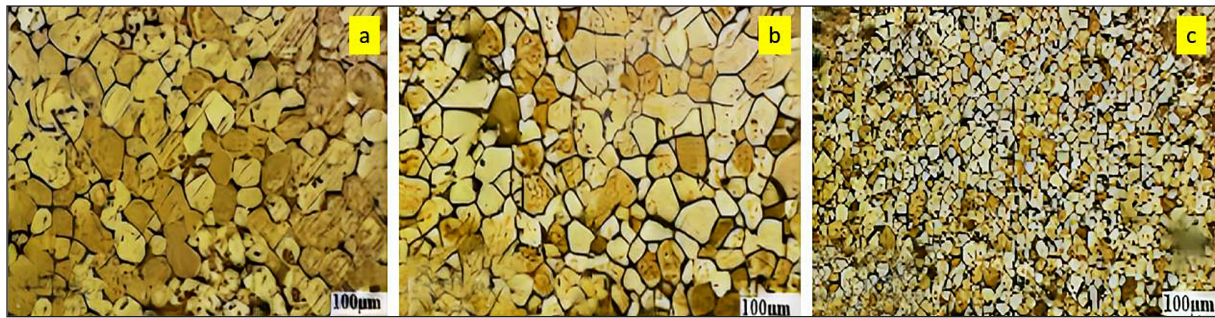
Figure 7. Optical microscope images of (a) original Al 6063 specimen, (b) extruded Al 6063 at 350 °C, (c) extruded Al 6063 at 500 °C. Mag: ×1000
