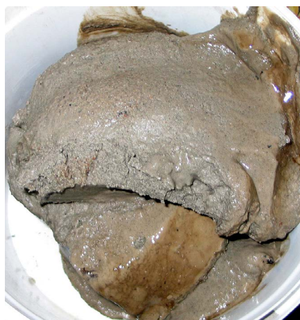
Phot. 2. Spoil sample (drill cuttings + drilling fluid)
