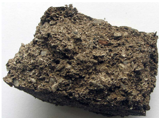
Phot. 6. The solidified sample of drilling-related waste from P-1 opening (binding additive 2.5% SCQ25 + 0.5% of sodium water glass)
