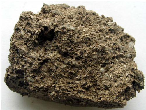
Phot. 7. The solidified sample of drilling-related waste from B-1 opening (binding additive 10.0% SCQ25 + 0.5% of sodium water glass)
