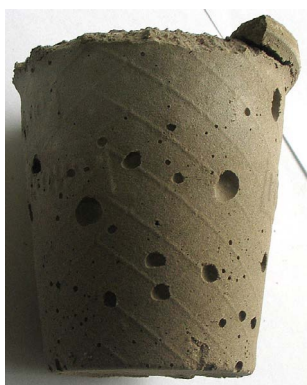
Phot. 5. The solidified sample of drilling-related waste from B-1 opening (binding additive 10.0% SCQ25 + 0.5% of sodium water glass)
