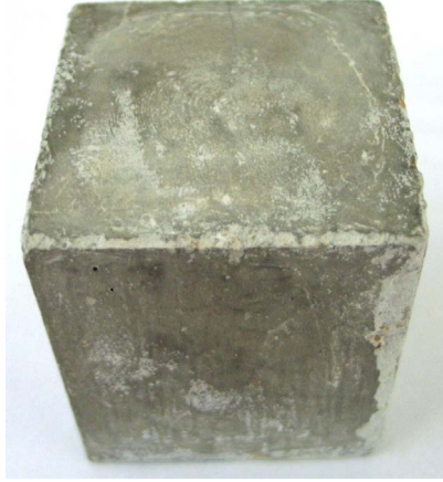
Phot. 3. The solidified sample of drilling-related waste
