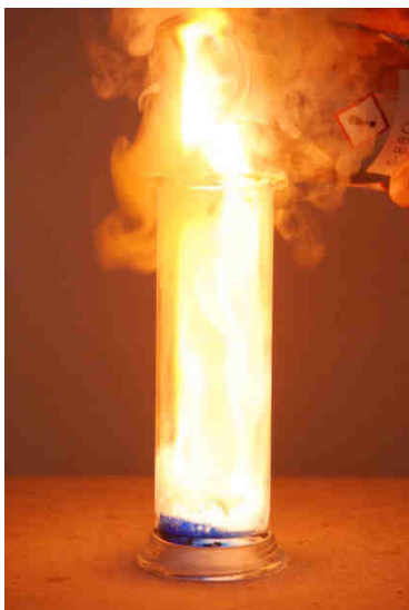
Photo 15. The spontaneous combustion of ammonia reacting with excess chlorine, and the appearance of the deep blue copper tetramine complex ion at the bottom of the gas jar
