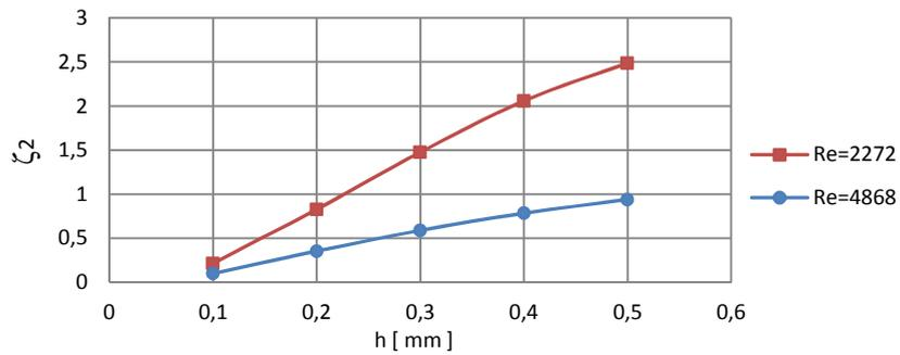
Fig. 9. IEC outlet local loss coefficient for laminar and turbulent flow
