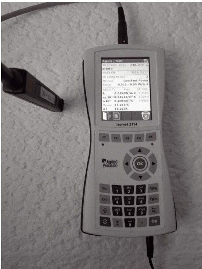
Figure 3. Investigations of the thermal properties of the insulating foam
