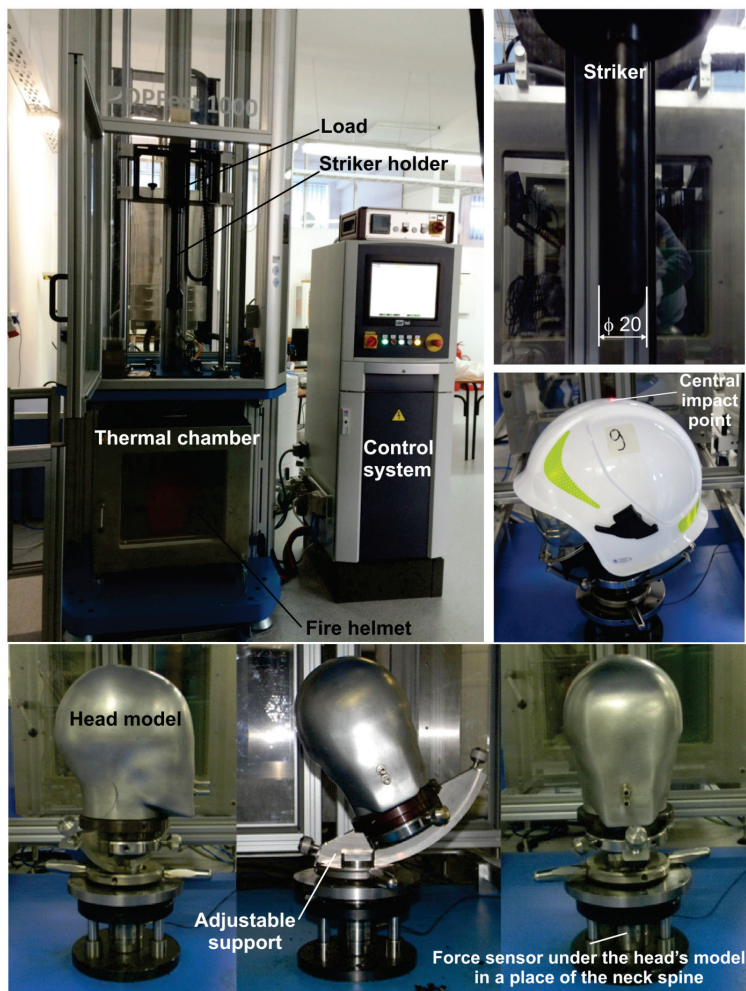
Fig. 1. Test stand for fire helmets testing under dynamic mechanical (impact) loads
