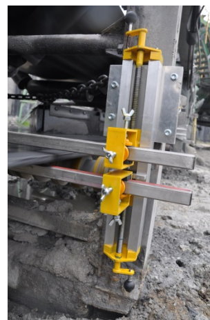
Fig. 2. Two permanent magnet bars mounted in the holder
