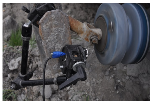
Fig. 4. Measurement of conveyor velocity with magnetic encoder
