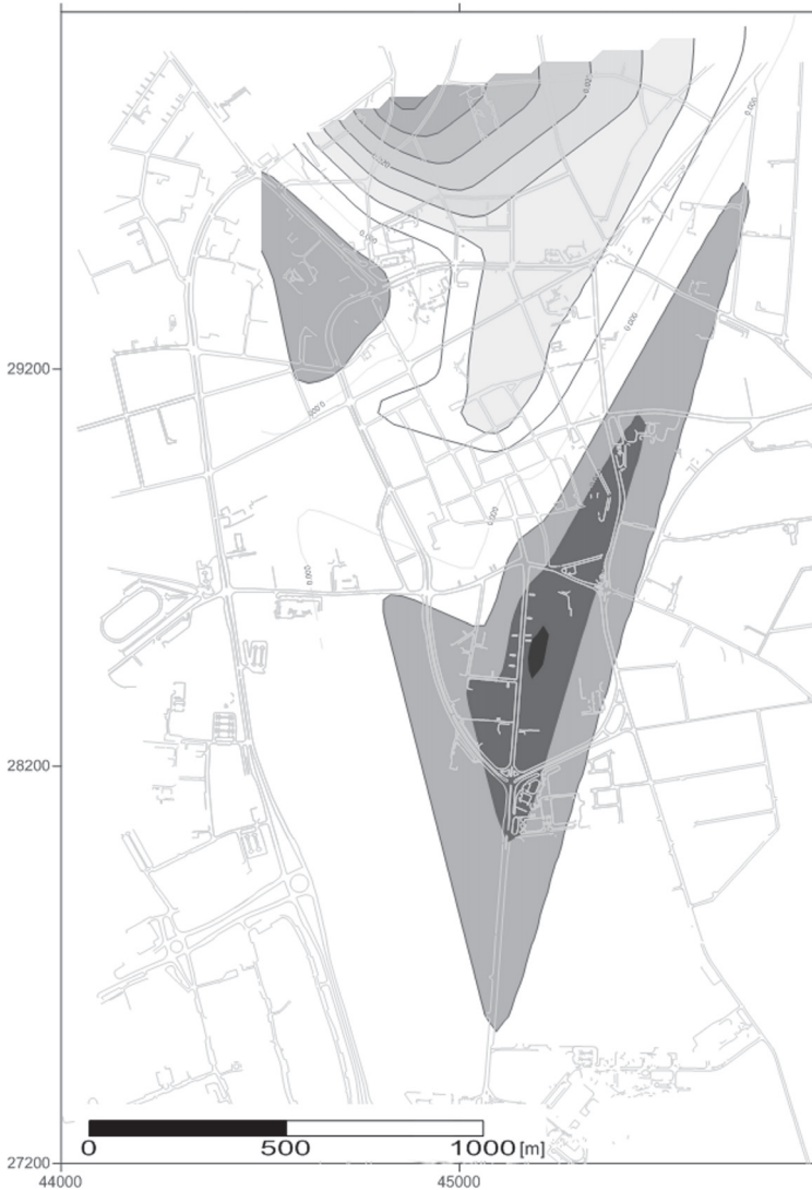
Fig. 2. The distribution of vertical displacements on the area of Inowrocław between 1992 and 2007
