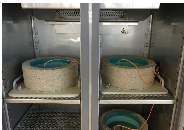
Figure 6 Samples stored in the climate chamber during the test
