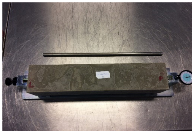
Figure 4 Determination of change in the sample length
