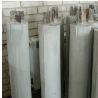
Fig. 5b. Pile specimens with I100 reinforcement
