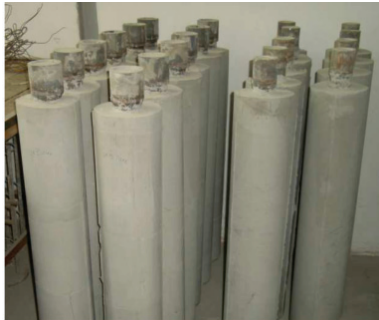
Fig. 5a. Pile specimens with steel tube reinforcement
