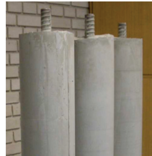
Fig. 5c. Pile specimens with SAS system rebars
