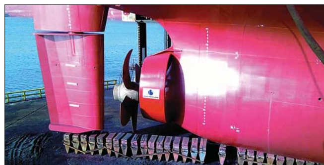
Fig. 1. The wake equalizing duct (Becker Mewis) installed on a -chemical tanker [1]
