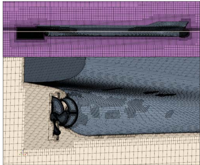
Fig. 4. Computational mesh for both ship and aft body of ship with propeller and duct
