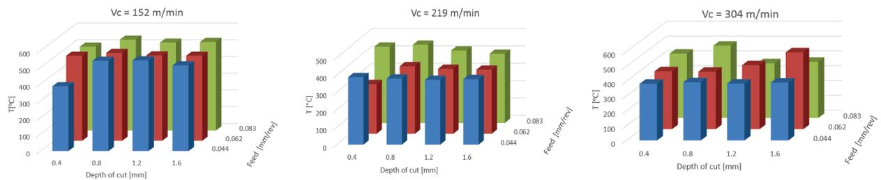
Fig. 6. The influence of changing of cutting parameters on  $T$  for  $V_c = 152, 219, 304$  m/min
