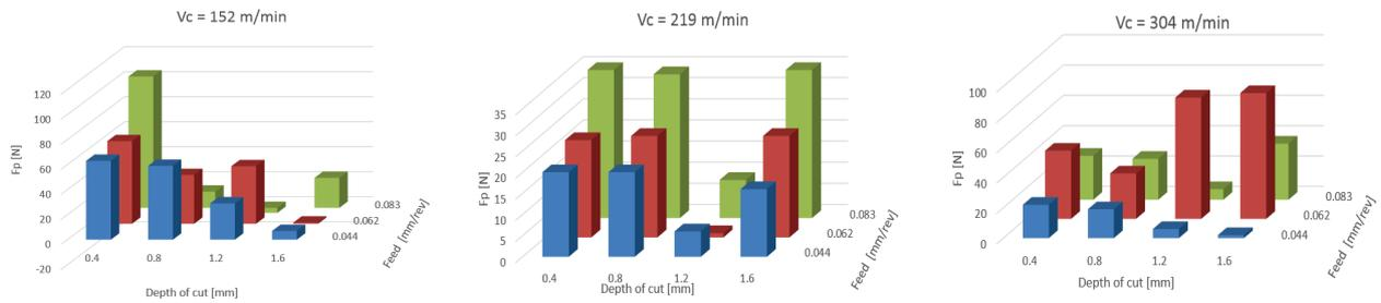
Fig. 5. The influence of changing of cutting parameters on  $F_p$  for  $V_c = 152, 219, 304$  m/min
