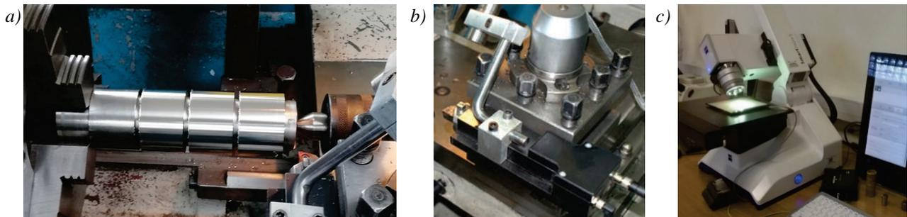
Fig. 1. a) The sample used for turning process, b) DKM 2010 turning dynamometer, c) Smart zoom 5 microscope
