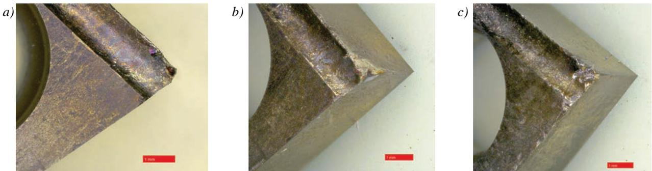
Fig. 7. View of insert: a, b) during turning process, c) after turning process
