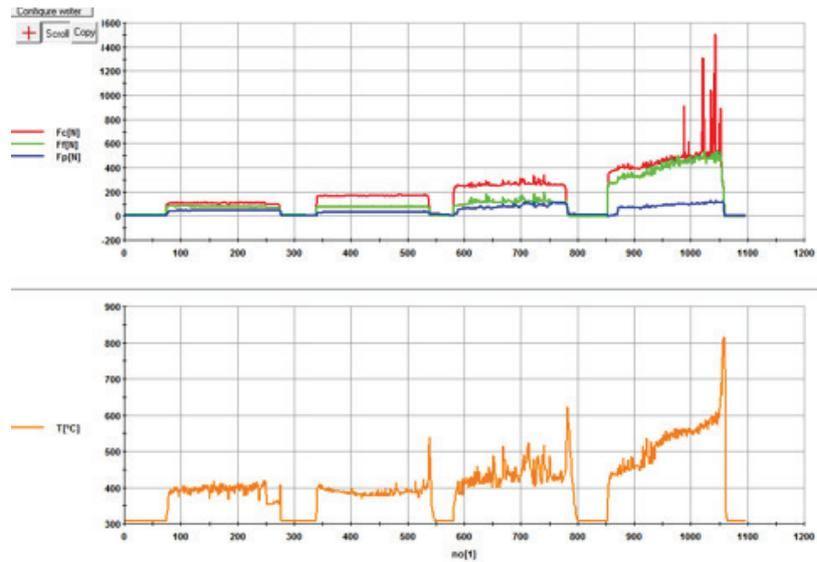
Fig. 2. Effect of change of cutting depth on value of cutting forces and temperature
