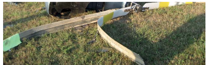
Fig. 1. Illustration of consequences resulting from delamination of a composite blade of helicopter lifting rotor during flight
