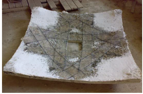
Fig. 6. Shell strengthened using 2-layers of glass fiber wrap (Type 3).
