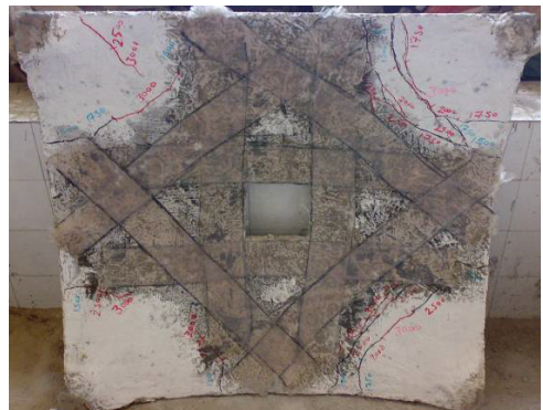
Fig. 22. Crack pattern of shell Strengthened by using 2 layers of GFRP (Type 3). [Failure load = 3500 kg]
