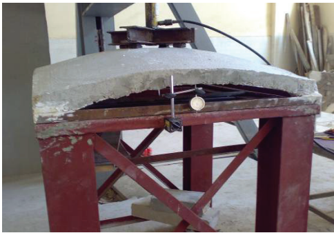
Fig. 7. Shell strengthened by using external tie.
