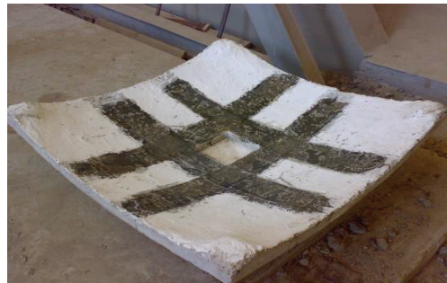
Fig. 4. Shell strengthened using 2-layers of glass fiber wrap (Type 1).
