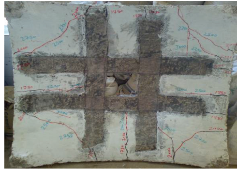
Fig. 24. Crack pattern of shell repaired by using 2 layers of GFRP (Type 1). [Failure load = 3000 kg]
