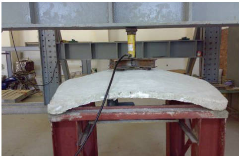
Fig. 3. The arrangement of the hydraulic jack which applying the load.
