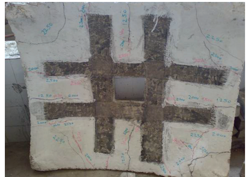
Fig. 20. Crack pattern of shell Strengthened by using 2 layers GFRP (Type 1). [Failure load = 3500 kg]
