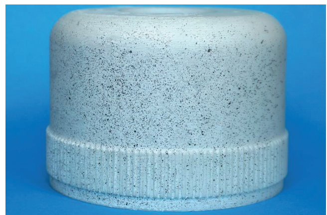
Fig. 3. Model of the flexspline, ready for optical measurements
