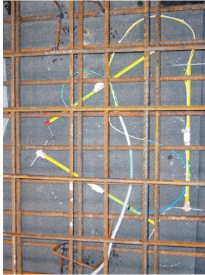
Fig. 4. A rosette installed in the area of the load of the wheels of the main left leg
