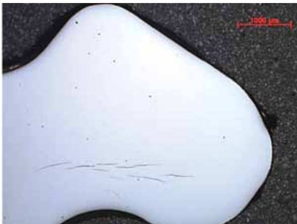
Fig. 8. Crosswise cross-section of the shape wire with visible micro cracks [11]
