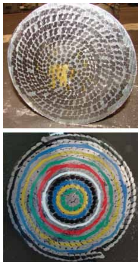
Fig. 6. The stay rope cross sections: after cutting off the thimble (left) and with the marked layers of wires to be included in the testing (right) [9]
