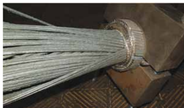
Fig. 7. The “broom effect” after cutting off the layers of the wires [9]
