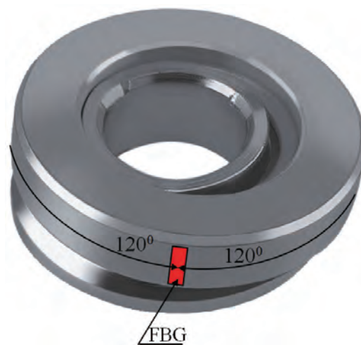
Fig. 6. Scheme of the intermediate bearing spherical pad with FBG sensor location
