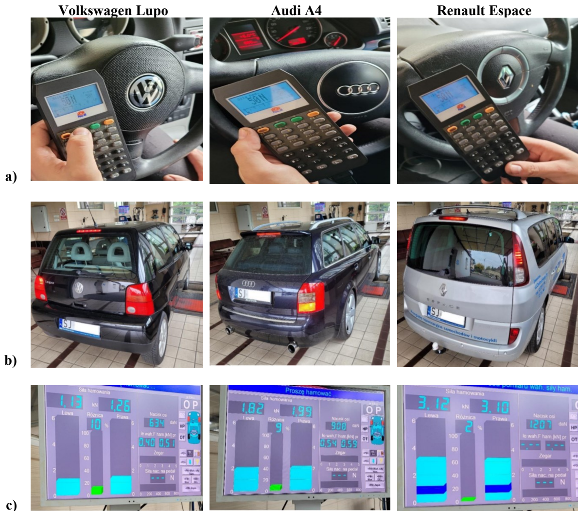
Figure 3. The course of the technical test of measuring the braking forces, a) setting the pressure of 50N on the brake pedal, b) measurements on a roller device, c) example measurement results.
