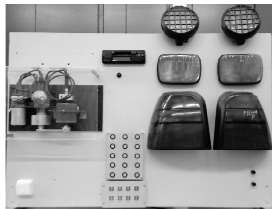
Fig. 2. View of main part of laboratory stand for the car electrical installation analysis
