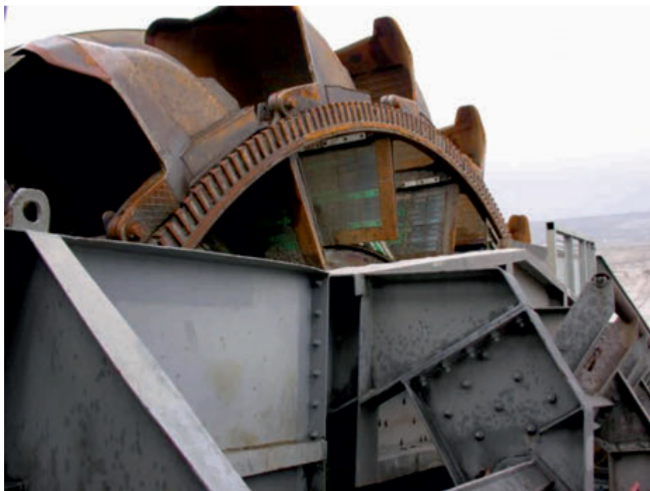
Fig. 5. Semi-cell bucket wheel of BWE SchRs 4000
