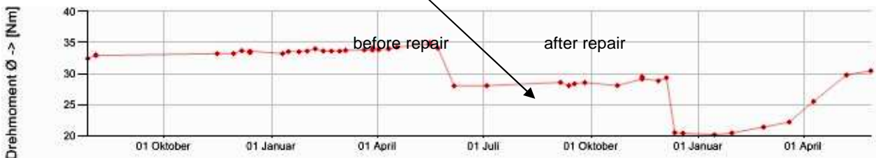
Test with constant velocity, vertical axes, Machine 3
