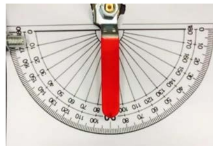
Fig. 3. Protractor instrument for measuring angles at suction valve of the pump.
