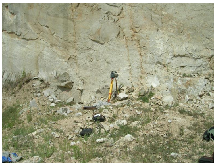
Fig.2. A portable gamma-ray spectrometry workstation GX3020 at location 1 (Kamienna Góra).
