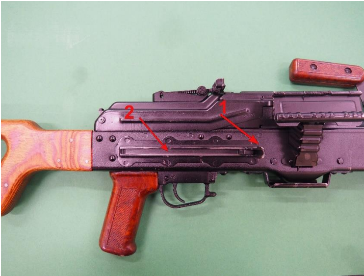
Photo 4. PKM general-purpose machine gun breech bolt receiver: 1 – carrier charging handle; 2 – guide
