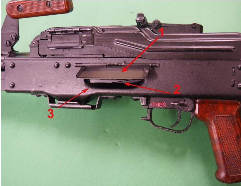
Photo 3. PKM general-purpose machine gun breech bolt receiver: 1 – case ejection port, shown open; 2 – dust shield opening lever, shown extended; 3 – bolt carrier assembly, shown moving forward
