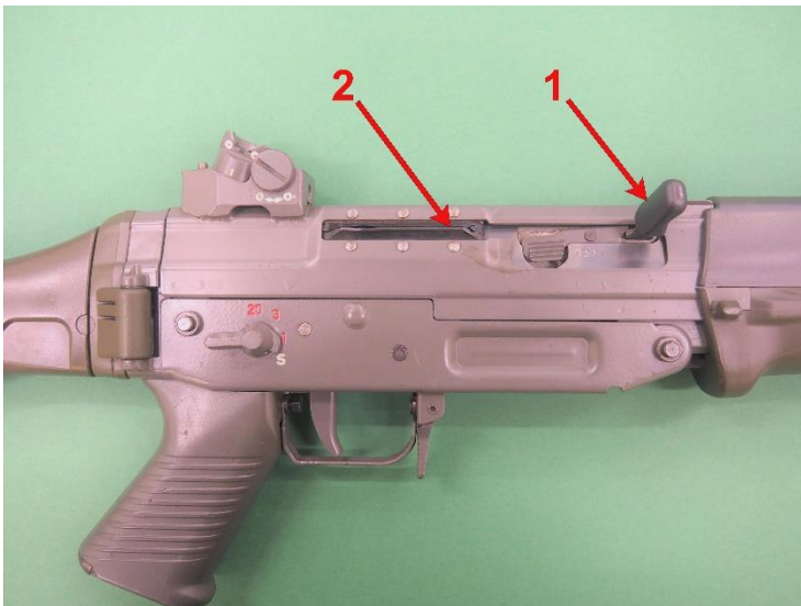
Photo 5. SIG 552 rifle upper receiver: 1 – carrier charging handle; 2 – guide
