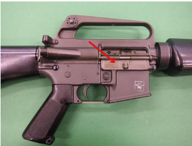
Photo 2. M16A1 rifle upper receiver: the case ejection port shield is shown open with the carrier charging handle
