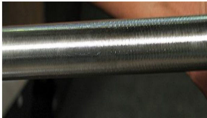
Fig. 11. Unstable machining, chatter
