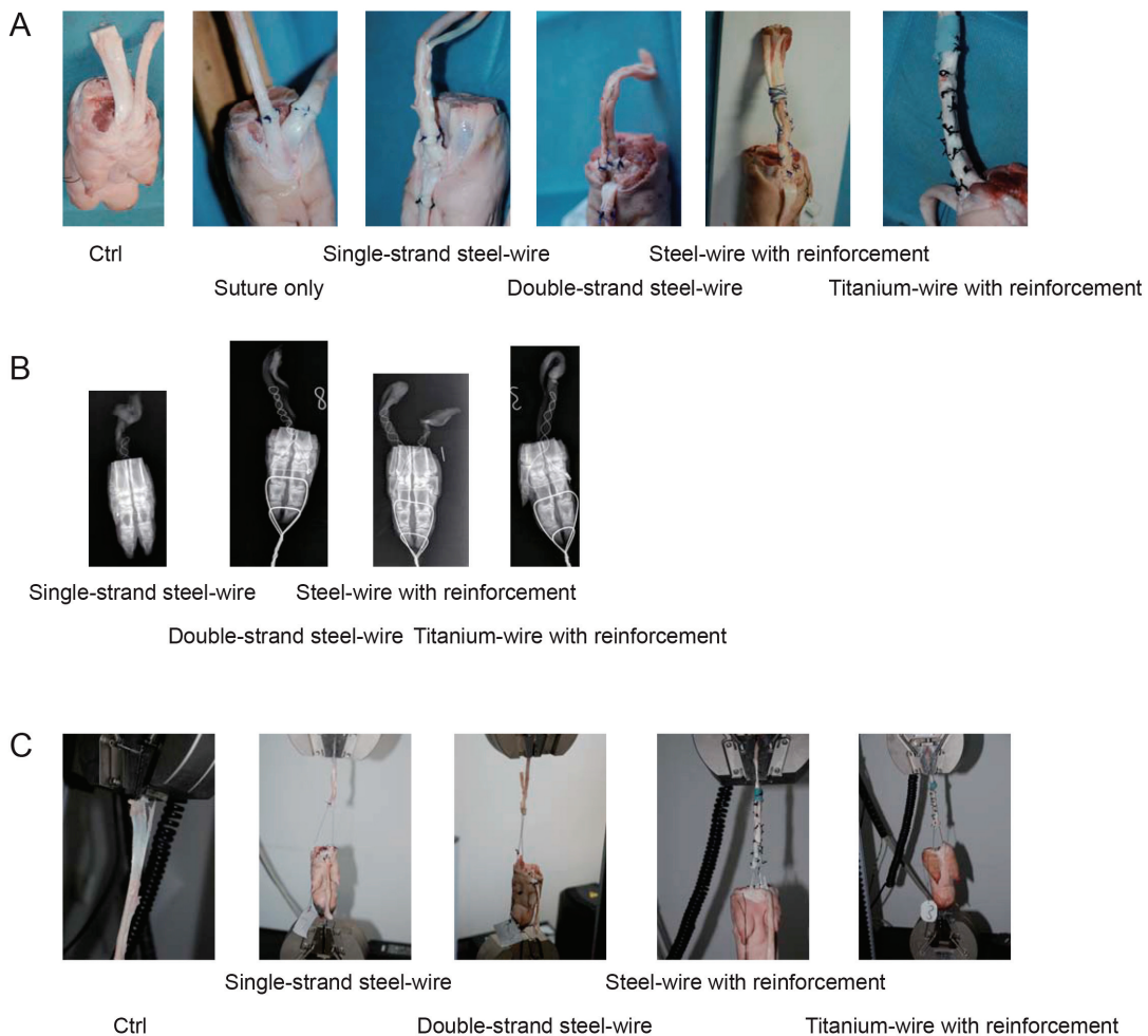
Fig. 3. Images of sutured tendons (A) and radiological pictures of tendons (B) in different groups as indicated. Figure 3C showed images of tendons at failure load in groups as indicated
