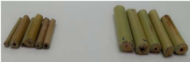
Fig. 2. Small and large diameter samples of bamboos.
