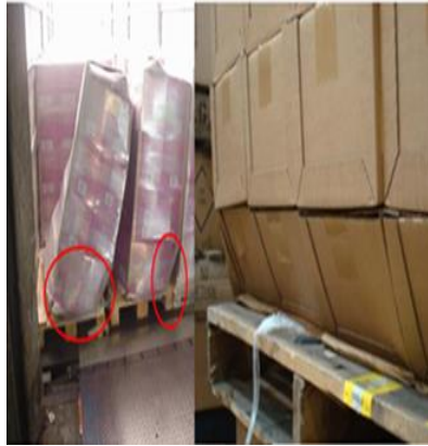
Fig. 11. Damage requiring re-packaging due to loss of physical properties (own pic.)
