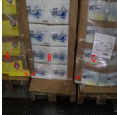
Fig. 6. Breaking off the load from the loading pallet (own pic.)
