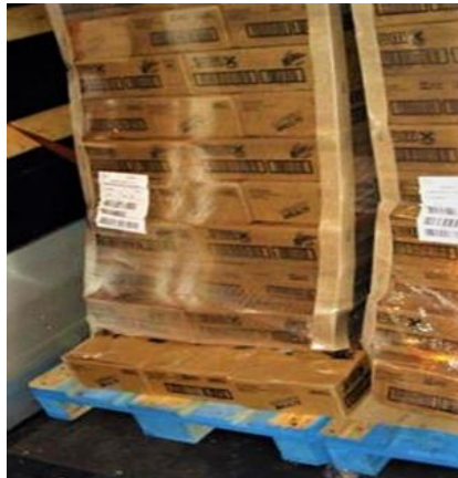
Fig. 3. Offset that slightly displaces the load outside the pallet area (own pic.)
