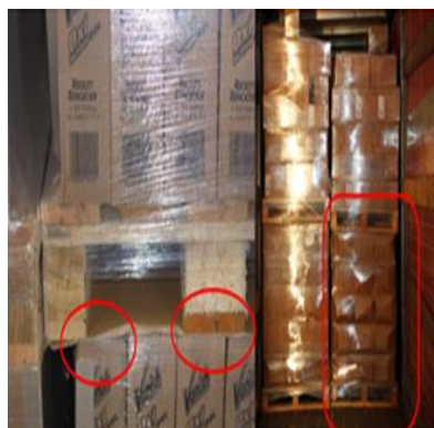
Fig.13. Damage to stacked loads (own pic.)
