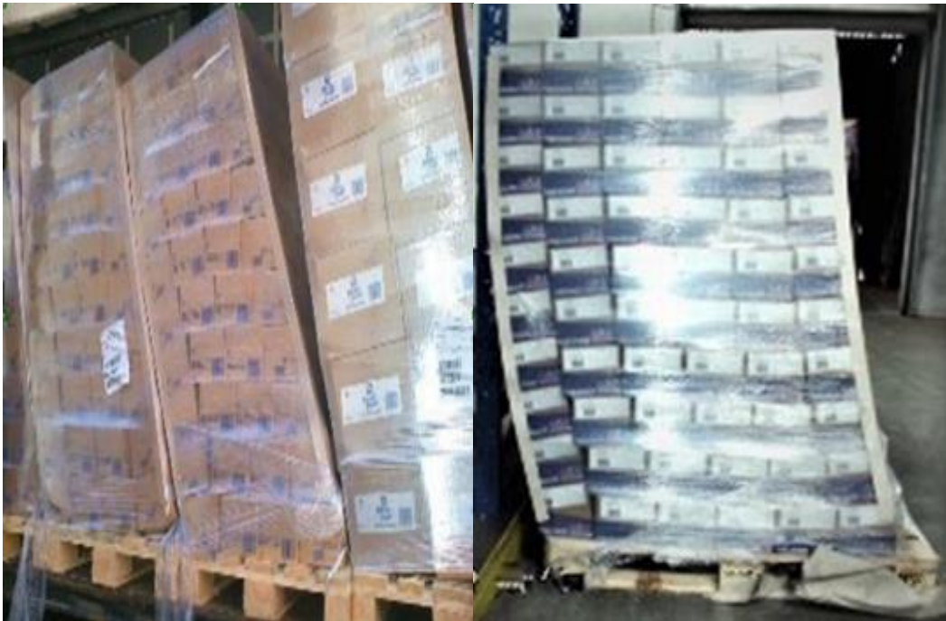
Fig. 5. Tilt significantly shifting the load behind the pallet area (own pic.)
