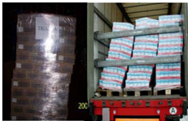
Fig. 8. Relaxing requiring the load to be rebuilt on the pallet (own pic.)
