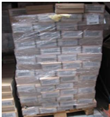
Fig. 7. Relaxing of the wrapping that requires reinforcement (own pic.)
