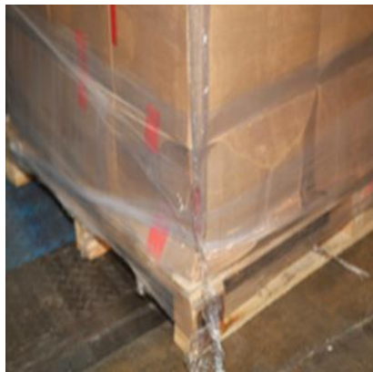
Fig. 9. Damage requiring local load strengthening (own pic.)
