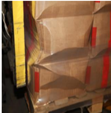
Fig. 10. Damage requiring building a new load and replacing the secondary packaging (own pic.)
