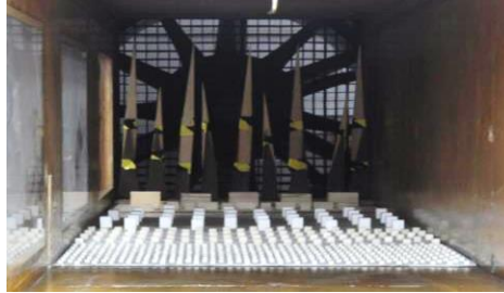
Fig. 2. Elements shaping the profile of velocity
