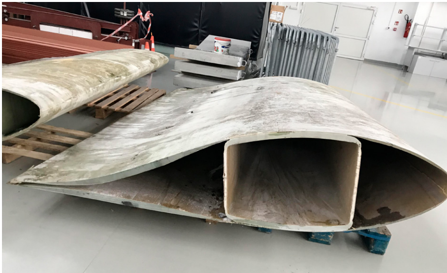
Figure 7. View of sections taken from wind turbine propellers
