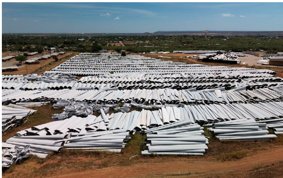
Figure 2. Discarded wind turbine blades fill thirty acres on the west side of Sweetwater Source: Doomberg, 2023.
