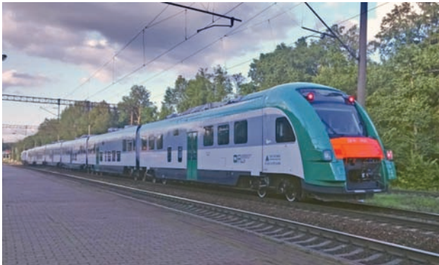
Fig. 11. DMU of the DP6/760M-006 series (Pesa, 1520 mm), BC railway, Minsk suburbs [photo S. Badionkin, 04.09.2020]
