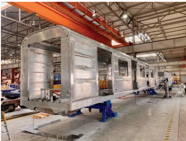
Fig. 15. Aluminium body for a Warsaw underground train [photo M. Tobrman / Škoda]
