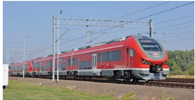
Fig. 12. DMU of the 633-001 series (Pesa) for DB Regio at the experimental track of the Railway Research Institute in Węglewo near Żmigród [photo M. Graff, 06.09.2018]
