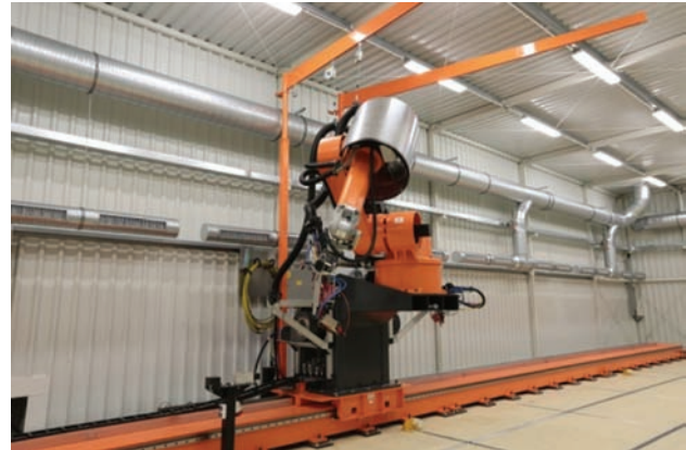
Fig. 3. Industrial robot for laser welding at the Bombardier plant in Wrocław [photo M. Kaczanowski / Bombardier, 07.06.2017]
