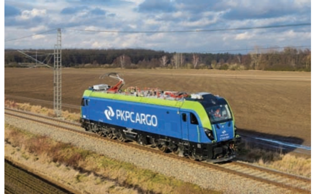
Fig. 6. A Dragon ET43-001 locomotive (Newag; 3 kV DC, 25 kV 50 Hz) during technical and operational tests on the experimental track in Cerhenice near Velim, Czech Republic [photo J. Navratil, 24.01.2021]
