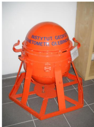
Fig. 3. Sea-bottom magnetometer for magnetic measurements at the Baltic Sea bottom. (Source: Marianiuk J. et al., 2007)
