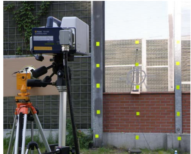
Fig. 9. Laser scanning vibrometer and investigated noise barrier. Distribution of measurement points.
