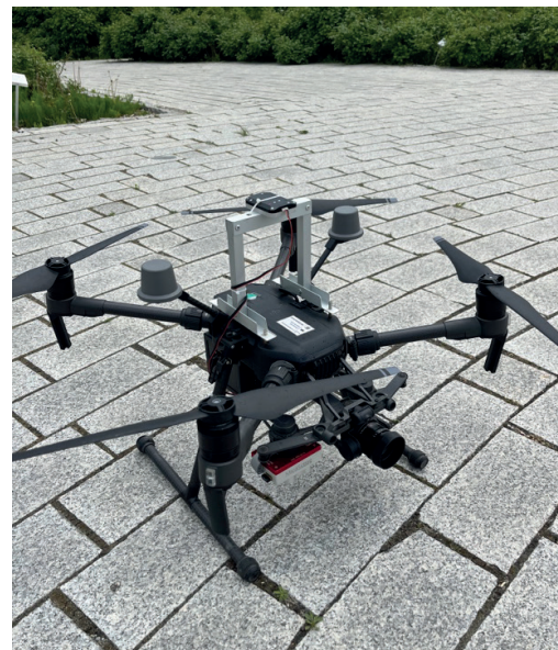
Fig. 3. Matrice 210 RTK v2 unmanned aerial vehicle used in the study, with the Micasense multispectral camera (left side) and X5S optical camera (right side) and DLS sensor (top of the drone) mounted
