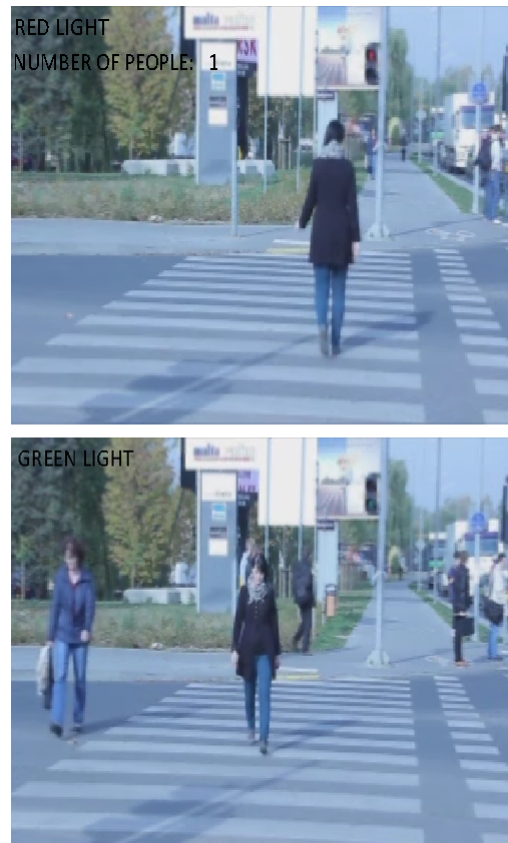
Fig. 13. Results of the people detection at red light on pedestrian crossing model performed with DM6437 EVM.
